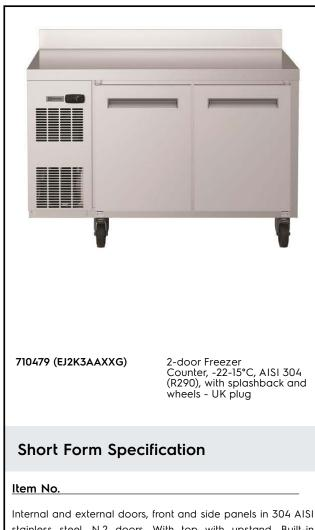
stainless steel. N.2 doors. With top with upstand. Built-in refrigeration unit. Ventilated. Refrigerant R290. High-density expanded polyurethane foam, 90 mm in thickness, with cyclopenthane injection. Digital control panel. Completely automatic defrosting and automatic evaporation of defrost water obtained by hot gas. Temperature range: -15/-22°C. CFC and HCFC free. Feet in 304 AISI stainless steel, adjustable in height. Delivered with wheels and with UK plug.
